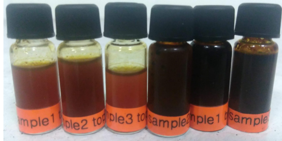
Figure 18 Top fraction (left) and bottom fraction (right) of pyrolysis oil from fiber.
